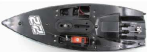
Hull installed with servos & battery box
